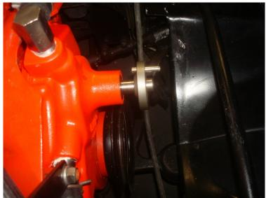
When installing these parts I use a quarter inch diameter by one inch dowel pin.
