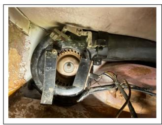
Here's an accurate depiction of the tight fit. Notice the combination trap door lever and fan two speed power switch at the top. Just above is the inside of your coupe body surface. In this photo, the wiring harness is not yet connected.
