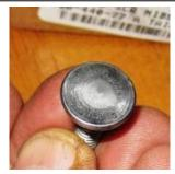
The exposed head of the weld stud looks very similar to a correct rivet head, and when painted with silver paint, is almost indistinguishable from a correct rivet. I'm sure there are at least a couple of judges who'd take issue with this, though;-)
