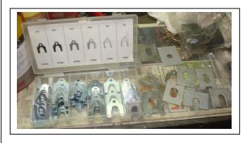
Joe directed me with the number or thickness of shims to raise the car at Body Mount 1 and 2. We raised both of these positions approximately 3/8 of an inch and I removed one thin shim at Body Mount 3.
