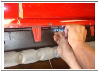
There is very little space between the body mount bracket and the body of the car. We had to remove a splash shield at the front body mount and used a bolt to hold the shims
