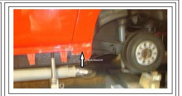
In effect we are positioning the front of the car along with the door to point up higher to align with the rear fender. We will use body shims to accomplish this.
