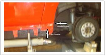
At this time the door was just a little bit low to the fender. So we loosen the bolts holding the door hinges and using wood shims under the door attempted to raise the rear just a little bit. The Door and the rear fender aligned perfect.
